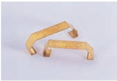
Couplings with rubber gaskets are likely to function as an insulator. Where electrical continuity is required, the Shurjoint continuity clip will restore electrical continuity to the system. The electrical continuity clip satisfies IEE Wiring Regulations. Material: Copper or Brass plate.
