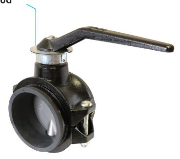
The Fig. 70G Butterfly Valve is designed for use with Gruvlok couplings, an ASC Engineered Solution, for fast and easy installation on grooved pipe. The valve body is fully rubber lined in EPDM or Nitrile material. A 316 Stainless Steel Disc is standard. The valve is supplied with a two position lockable handle.
