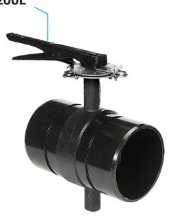
Model B8200L Butterfly Valves are available in sizes 2 through 8 inch diameters. Precision machined grooves in the valve body provide easy alignment of the valve and compatible PVC couplings, allowing for the insertion of the spline to connect the Model B8200L Valve to the PVC piping system. Flow may enter the valve from either direction and valve can be orientated in any direction.
