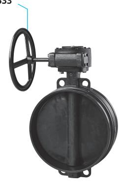
The Model B333 Large Diameter Butterfly Valve provides efficient control of fluid flow in piping systems. It is a grooved-end bubble tight shut-off valve with end-to-end dimensions that meet MSS SP-67, Table 4 and a mounting pad that meets ISO 5211 for the mounting of power actuators. The valve is capable of bidirectional fluid flow at working pressures to 300 psi (20 bar) and may be positioned in any orientation.
