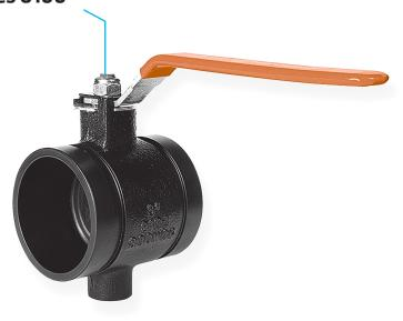
The Series 8100 Low Profile Butterfly Valve has a rated working pressure of 300 psi (20.7 bar) and provides efficient control of fluid in piping systems. Flow can be from either direction and the valve may be positioned in any orientation. The ductile iron body is epoxy-coated to resist atmospheric corrosion. The disc is EPDM encapsulated ductile iron compatible with a variety of chemicals and temperature ranges.
