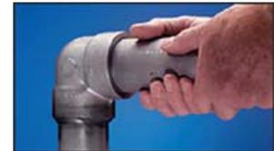
**3.** Fitter inserts pipe into fitting. Gap-A-Let® ring automatically assures the required minimum gap (1/16") to meet the code requirements of ANSI 31.1 Section III, ASME & military codes.
