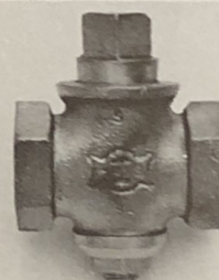
No. 7305 High Pressure Stop for Steam, Water, Gas, Oil, and Air. Working pressure up to 250 pounds. Bronze steam metal construction. Square head 1/2" thru 1 1/2".
