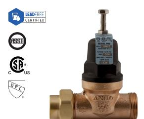
The Apollo 36ELF is designed for residential and commercial applications to protect water supplies from excessive pressure. Excellent flow performance at low pressure drop. The dezincification resistant bronze body and dielectric polymer cage provide maximum corrosion resistance. Designed for easy in-line servicing with simple cartridge removal. They meet ASSE 1003 and CSA B356 standards. They are listed with IAPMO and the city of Los Angeles.
