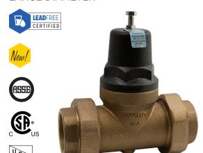
The new large diameter Apollo 36ELF Lead Free Pressure Reducing Valve is designed to conserve water and protect water distribution systems by automatically reducing elevated supply pressures. The dezincification resistant bronze body, stainless steel adjusting screw and dielectric polymer cage provide maximum corrosion resistance. Designed for easy inline servicing with simple cartridge removal.
